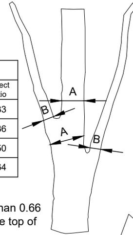
Aspect ratio of B:A less than 0.66 as measured 1" above the top of the branch union.
