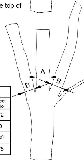
Aspect ratio of B:A greater than or equal to 0.66 as measured 1" above the top of the branch union.
