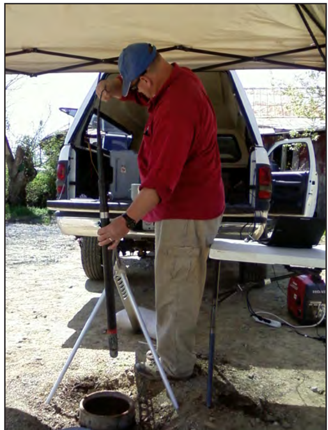
Figure 17. A gamma logging tool is inserted into a water-supply well in Hopkins County to help determine the rock type of the aquifer, since no driller's log was available for the well.
