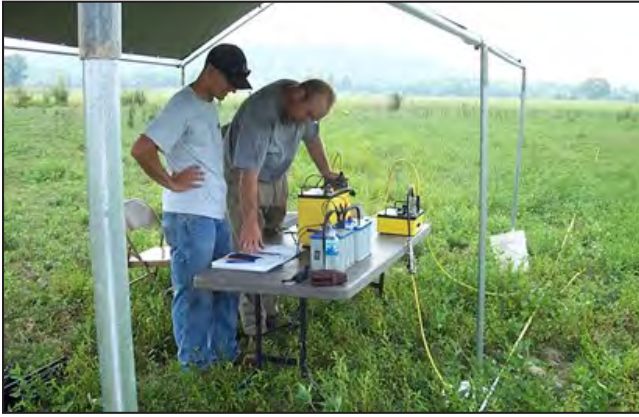
Figure 11. USGS scientists conduct a two-dimensional geophysical investigation of the groundwater near West Point, Ky.
